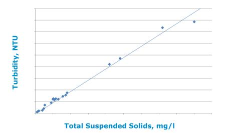
The Compact Turbimeter allows the insertion of a site specific relationship between the two parameters, either as a factor or from correlated data, and subsequent use of the calibration for measurement of Total Suspended Solids (TSS).
