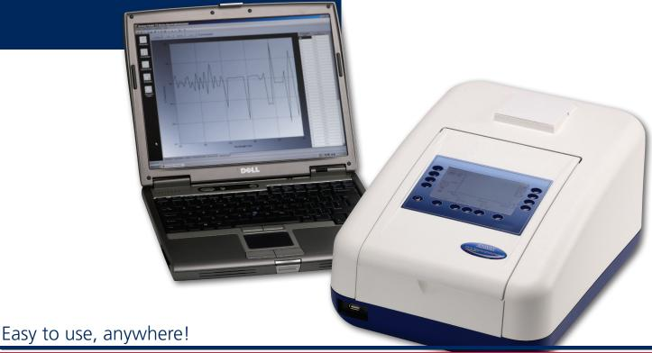
Through RS232 connection to PC, the software provides full emulation of all the instrument's functions and enables the instrument to be directly driven from a PC. The PC software also enables any optional accessories to be driven from a PC.
