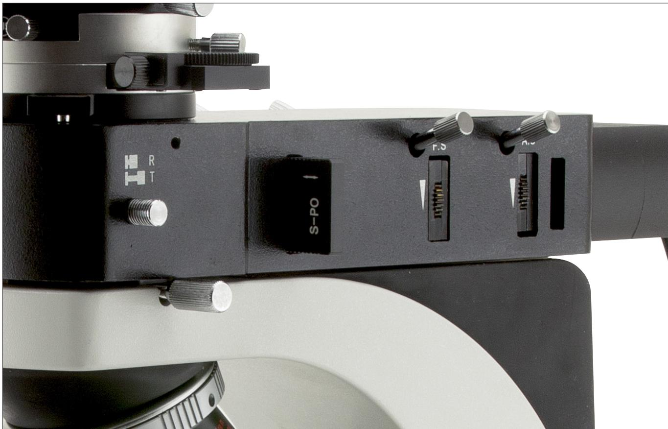
The analyzer filter can be inserted by means of the slider at the right side of the Bertrand lens attachment. The analyzer has a rotatable knob with a vernier scale engraved. For the "crossed Nicol" position put the scale in the "0" position.
