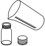
Fill a clean and dry vial up to the mark with Dilution Water (see chapter 2.3.7.1 Preparing Dilution Water).
