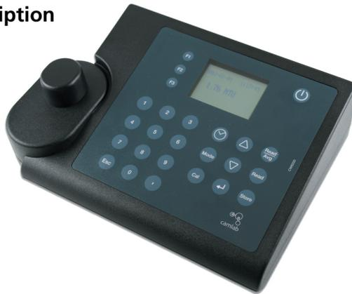
The CW8200 is a portable turbidity meter, based on the requirements of ISO 7027 (Water Quality – Determination of Turbidity). The instrument works with rechargeable batteries as well as with mains. As soon as the CW8200 is connected with the adapter to the mains the batteries are charged.
