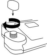
Rotate the vial in the sample chamber about 45°.
