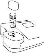
Place the vial in the sample chamber making sure that the positioning is correct.
