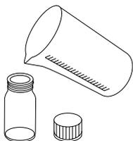
Fill a clean and dry vial with the water sample up to the mark (approx. 12 ml).
