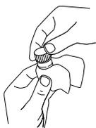
Take care to handle the vial by the top. Wipe the vial with a smooth and lint-free cloth to remove waterdrops and finger prints.
