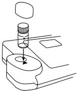
Place the vial in the sample chamber making sure that the marks are aligned.
