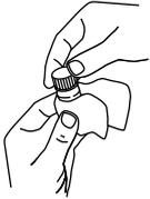
Hold the vial by the cap and wipe with a smooth, lint-free cloth to remove water spots and finger prints.
