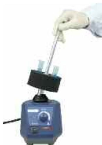
MX-S vortex mixer with 1189985 tube adapter holding rod
