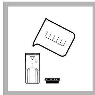
8. **Prepare the sample:** Fill a second 1-cm/10-mL sample cell to the 5-mL mark with sample.
