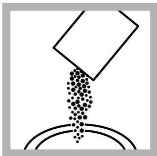
9. Add two 10-mL DPD Free Chlorine Reagent Powder Pillows or two 10-mL DPD Total Chlorine Reagent Powder Pillows to the second sample cell.
