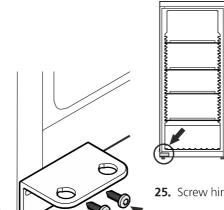
25. Screw hinge bracket into place.
