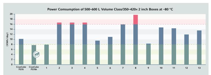
A comparison of the number of kilowatt hours per day it takes to keep 350 - 420 individual 2 inch boxes at a temperature of -80 °C in freezers with a volume of 500-600 L. The CryoCube F570h (230 V/50 Hz) can maintain the storage temperature using 7.6 KWh/day, less than 50 % of the energy required by some other units.
