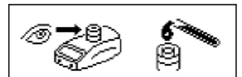
Check burner head (6) for clogging
