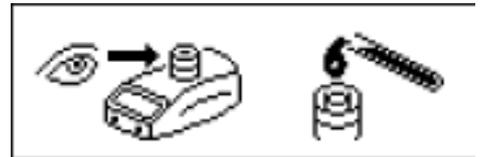
Check the burner head (6) for clogging
