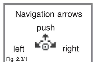
The arrows on the Display indicate in which direction the next menu items are accessible. If a submenu is selected by pushing the knob, the arrow blinks and also the parameter or alternatively the time which is to be set. The parameter or time can now be varied by turning the function knob.
