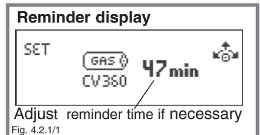
**(i)** The reminder occurs only after the previously set cartridge burning time has expired **and** the next time the flame is extinguished, i.e.: current use of the burner is not interrupted by the reminder. This may lead to inaccurate times in the event of long burning times.
