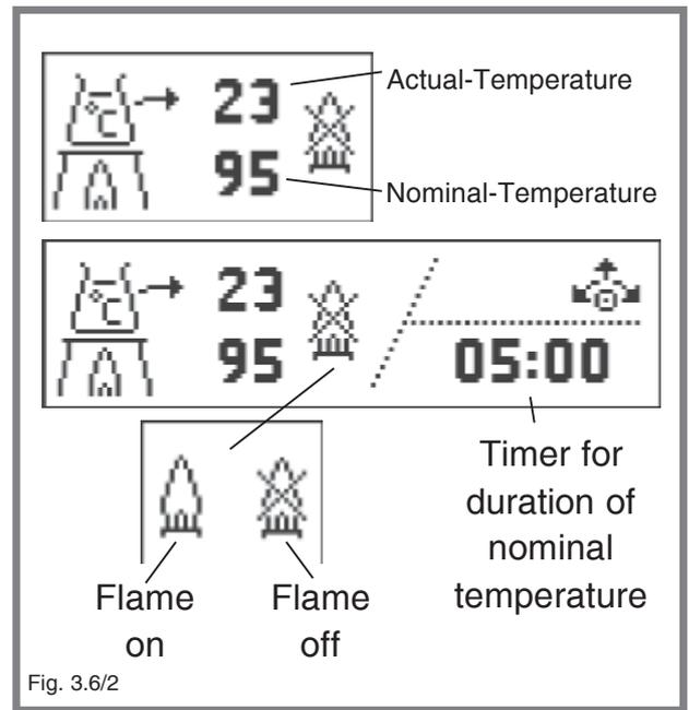
The temperature regulation program finishes when the nominal temperature has been reached and the timer period has expired.
