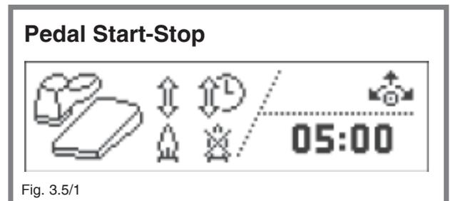
**i** This application program can only be used if the foot pedal is connected. To switch over from the application program Pedal Start - Stop to another program, turn the function knob **(1)** to the right or to the left.
