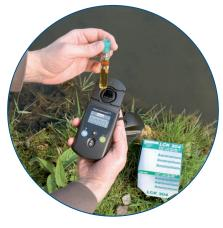
During this waiting time, the POCKET is set to zero using the blank value cuvettes supplied. All it takes is the touch of a button. The POCKET is then ready to measure the sample cuvette.
