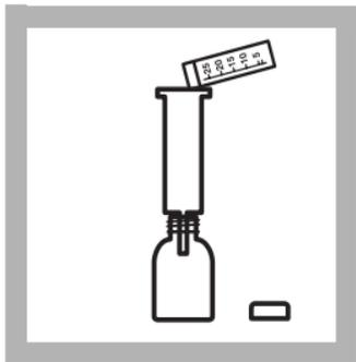
7. Place the extractor on top of the round poly mixing bottle. Measure 25 mL of pPb-3 Eluant Solution with the measuring vial and pour into the extractor.
