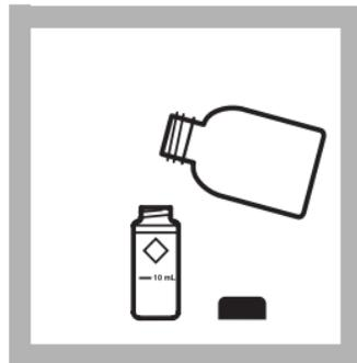
12. Fill a 10-mL sample cell to the 10-mL line with the prepared sample.
