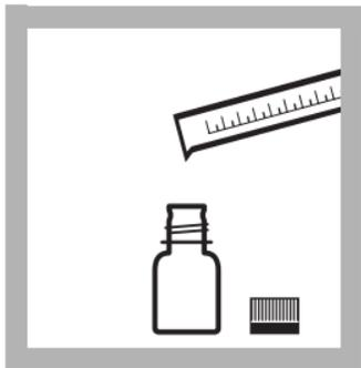
1. Fill a 100-mL plastic graduated cylinder with 100 mL of sample. Pour the measured sample into a 125-mL plastic sampling bottle.
