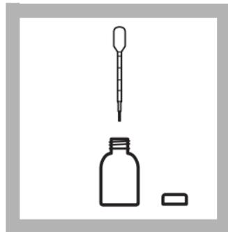
9. Remove the extractor from the bottle and, using a 1.0-mL plastic dropper, add 1.0 mL of pPb-4 Neutralizer Solution to the sample in the bottle. Swirl to mix thoroughly.
