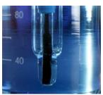
Owing to the ceramic junction, stable results for liquid samples are ensured.
