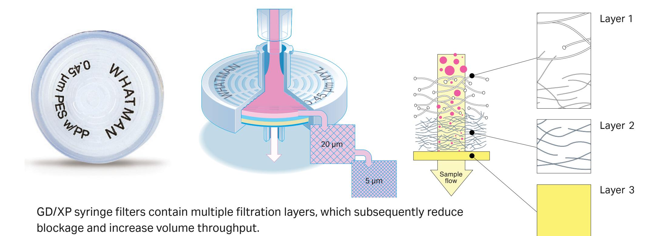
GD/XP syringe filters contain multiple filtration layers, which subsequently reduce blockage and increase volume throughput.
