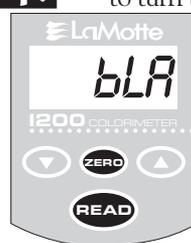
Push the **READ** button to turn the meter on. Press the **ZERO** button and hold it for 2 seconds until **BLA** is displayed. Release the button to take a blank reading (0.0 ppm).
