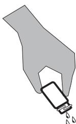
Rinse and fill a colorimeter tube (0290) to the 10 mL line with sample water. Cap and wipe dry.
