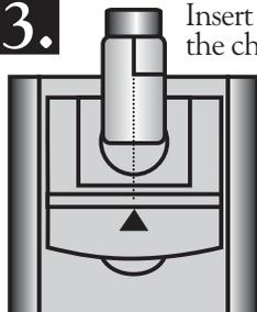
Insert the tube into the chamber, being sure to align the index line with the arrow on the meter. Close the lid. This tube is the blank or zero.
