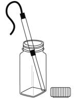
Close the digestion vial tightly with the cap and swirl until the reagent is dissolved completely.
