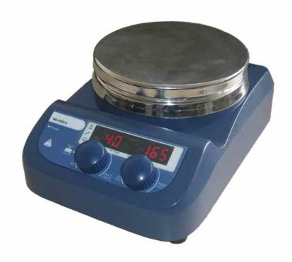
The Camlab Choice MS-H280-Pro is a small bench top magnetic hotplate stirrer that heats up to 280°C. It has a 135mm stainless steel hotplate with excellent corrosion resistance. The unit can be fitted with an external temperature sensor PT1000 for real time accuracy of +/- 1°C. The temperature and speed are displayed clearly by the LED panel. HOT warning indicates residual hotplate temperature after use.
