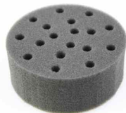
VT1.3.2 Tube adaptor 18 holes 10mm diameter
