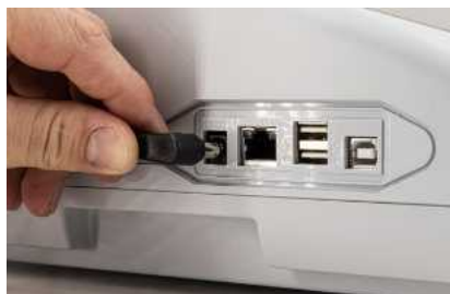
Fig. 2: Connecting the power supply
