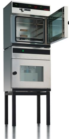
The direct contact between the load and the heatable and removable thermoshelves in the chamber of the Memmert vacuum oven ensures rapid and uniform temperature control of food, cosmetics, watches, books, PCBs or injection moulds, without the loss of heat.
