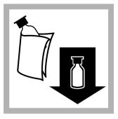
**10.** Within one minute after the timer expires, wipe the Ampul and insert into the cell holder.
