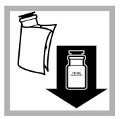
**10.** Within one minute after the timer expires, wipe the prepared sample and insert it into the cell holder.
