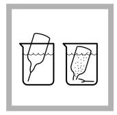
3. Tap the bottom of a NitraVer 5 Nitrate AccuVac® Ampul on a hard surface to dislodge powder. Fill the Ampul with sample. Keep the tip immersed while the Ampul fills completely. Insert a cap over the Ampul tip.
