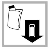
**8.** Wipe the blank and insert it into the cell holder.
