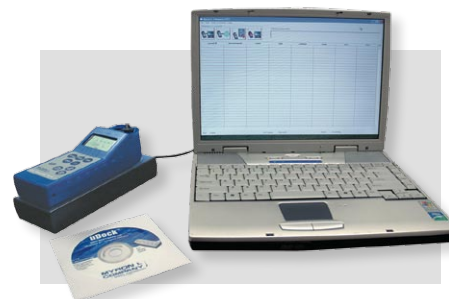
uDock™ in Action. U2CIP includes uDock, USB cable, and application software for your Mac or PC
