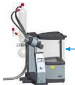
Protective cover for heating bath
