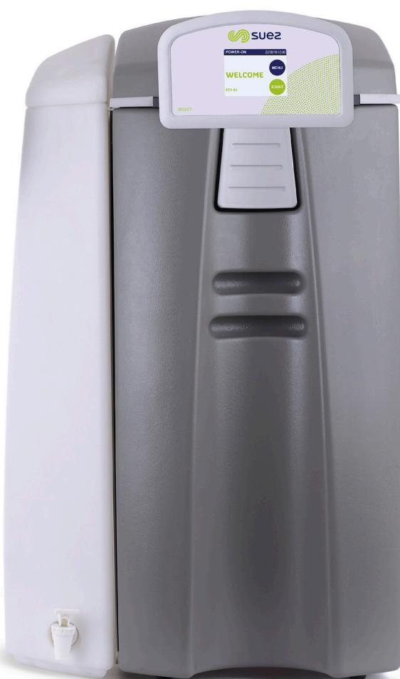
The Select edi 60 is a compact unit ideal for laboratory use delivering a constant supply of >5MΩ.cm pure water for laboratory tasks using activated carbon pre-treatment, double pass reverse osmosis, carbon dioxide membrane degassing and electro-deionisation technology.
