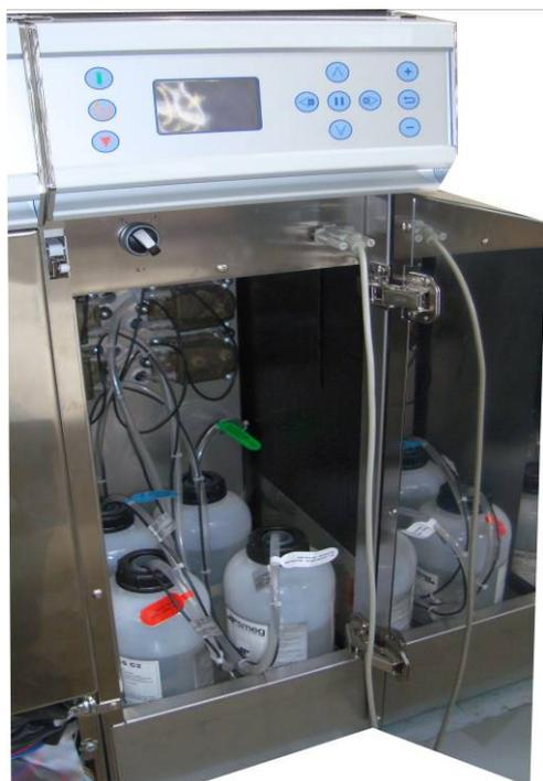
(NB: The detergent and acid containers are normally external to the machine!)
