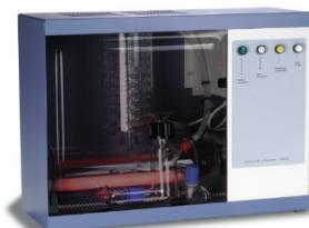
respectively, while the model A4000D produces 4 litres/h of double distilled water for more demanding applications. The reservoir level control automatically switches off the still when the collection vessel is full and re-starts it again once the distilled water is used. The Aquatron® can also be fed by a pre-treated supply such as a deioniser or RO unit to avoid the need to descale the still and improve the water quality.
