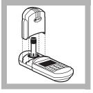
**19.** Place the "control" vial in the cell holder. Tightly cover the vial with the instrument cap. Record the absorbance value of the control.
