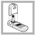
**20.** Place each sample or dilution vial in the cell holder. Tightly cover the vial with the instrument cap. Record each absorbance value.
