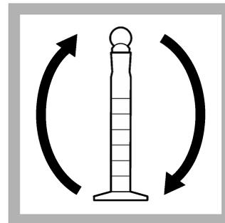
**4.** Close the cylinder. Invert the cylinder several times to dissolve the powder completely. Inconsistent readings may result if all the particles are not dissolved.
