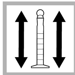
**8.** During the reaction period, close the mixing cylinder and vigorously shake the prepared sample. The sample becomes reddish-orange, brown or blue. The color is dependent on the zinc concentration.
