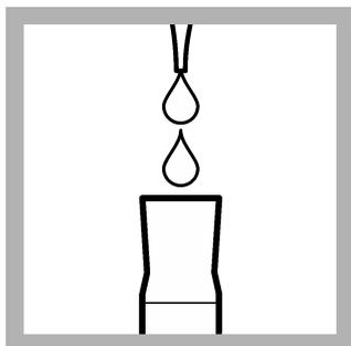
**6. Prepared the sample:** Use a plastic dropper to add 0.5 mL of cyclohexanone to the solution in the mixing cylinder.
