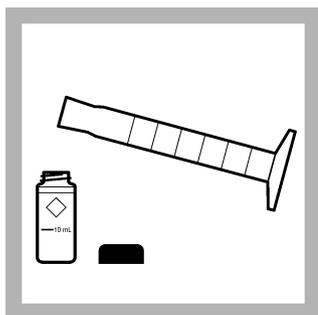
**10.** Fill a sample cell to the 10-mL mark with the prepared sample solution.
