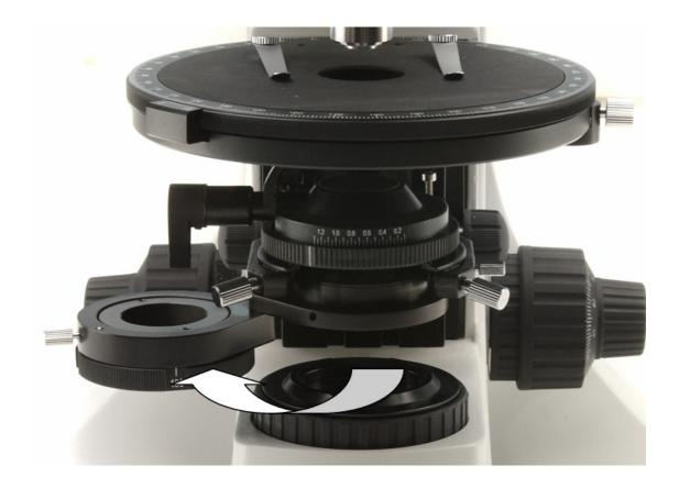
The analyzer filter can be inserted by means of its lever under the observation head. By holding this lever, it can laso be rotated at any angle:
