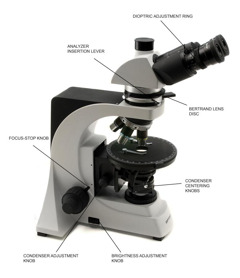
This microscope is a scientific precision instrument designed to last for many years with a minimum of maintenance. It is built to high optical and mechanical standards and to withstand daily laboratory use.
