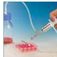
Aspiration with reverse modus valve
