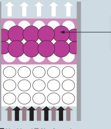
The violet filter layer of the new Dualfilter SealMax seals: No liquid passes through the filter. Both filter layers violet and white—retain aerosols and biomolecules reliably.
