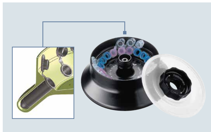
Eppendorf Kit rotor for 18 × spin columns and 1.5/2.0 mL tubes for speed up to 18,111 \times g/15,000 rpm. This rotor is designed with an extended rim that protects tube caps from shearing off (FA-45-18-11-Kit; Order no. 5424 706.002).
