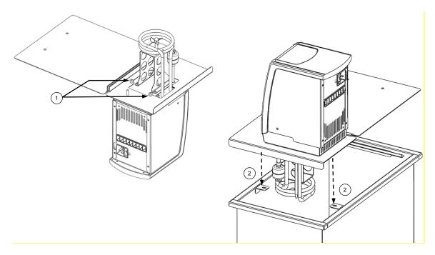
3. Fit the circulation tray in the base of the MST20 tank.
