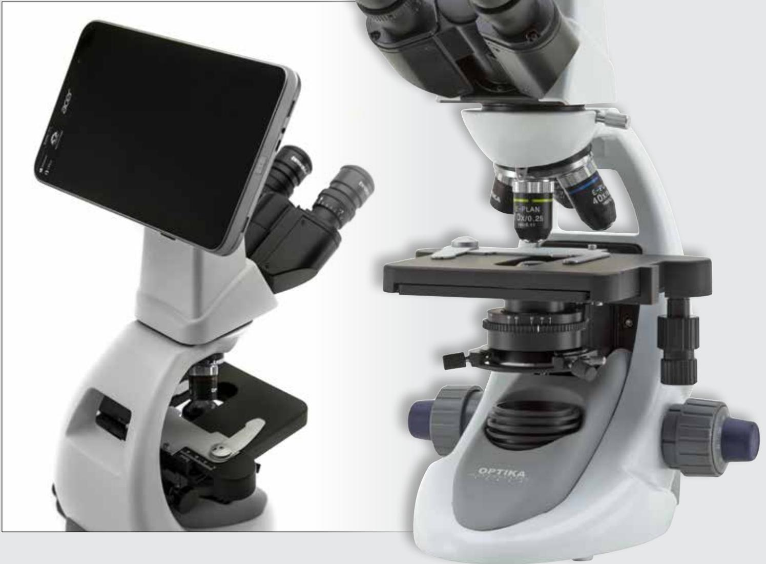
**Stand:** The stand has a modern and ergonomic design. It is easy to move the microscope thanks to the large opening behind the revolving nosepiece, to be used as a handle. The opening allows the user to see clearly the objectives and the samples, as requested in discussion groups.
