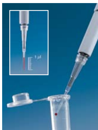
Transferpette® 0.1-1 µl with nano-cap™ pipette tip
