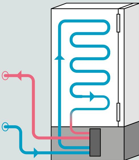
You can improve the conditions and comfort in your lab while saving energy by installing a water-cooled Eppendorf freezer. Many ULT freezers use the air in the laboratory to extract heat energy from the freezer's heat exchanger. Another option is to use a water-cooled ULT freezer connected to a facility's recirculating water system. A constant stream of water removes the heat from the heat exchanger, rather than the ambient air in the lab.
