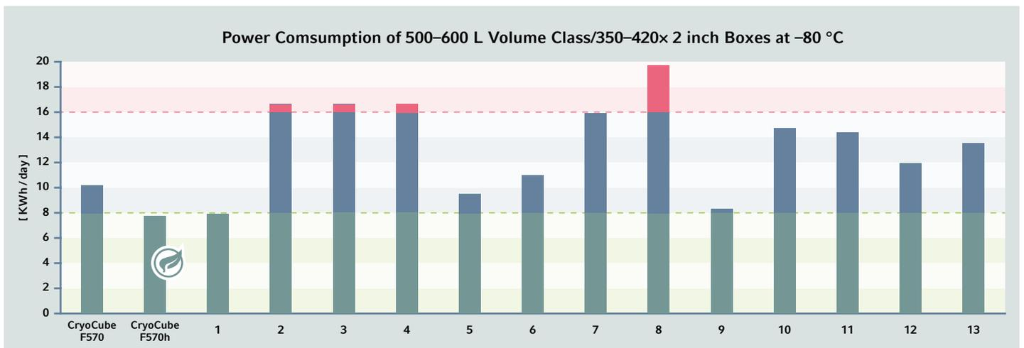
A comparison of the number of kilowatt hours per day it takes to keep 350 – 420 individual 2 inch boxes at a temperature of -80 °C in freezers with a volume of 500–600 L. The CryoCube F570h (230 V/50 Hz) can maintain the storage temperature using 7.6 kWh/day, less than 50 % of the energy required by some other units.
