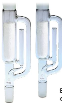
Extraction thimbles in Soxhlet extraction apparatus
