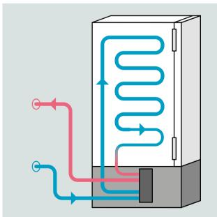
You can improve the conditions and comfort in your lab while saving energy by installing a water-cooled Eppendorf freezer. Many ULT freezers use the air in the laboratory to extract heat energy from the freezer's heat exchanger. Another option is to use a water-cooled ULT freezer connected to a facility's recirculating water system. A constant stream of water removes the heat from the heat exchanger, rather than the ambient air in the lab.
