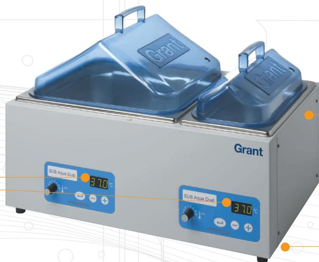
Fixed thermal cut-out – protects the user if the bath is accidentally run without water, or in the very unlikely event of failure of both control systems
