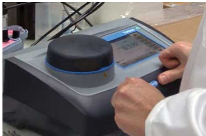
Figure 4: TU5200 installation in a French drinking water plant
