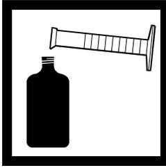
**2.** Using a clean graduated cylinder, pour the correct sample volume into a BODTrak sample bottle (see *Table 5*). See section 4.2 *Sample Dilutions* for more information on BOD range selection.
