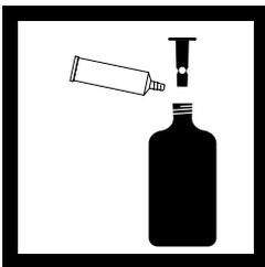
**5.** Apply Stopcock Grease to the seal lip of each bottle and to the top of each seal cup.
