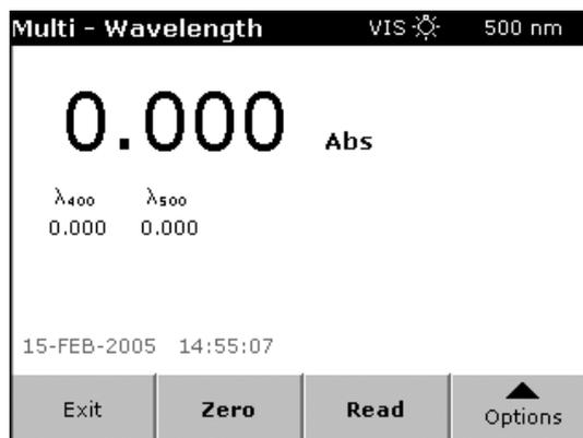
**Note:** The **READ** key does not become active until the zero measurement has been completed.
