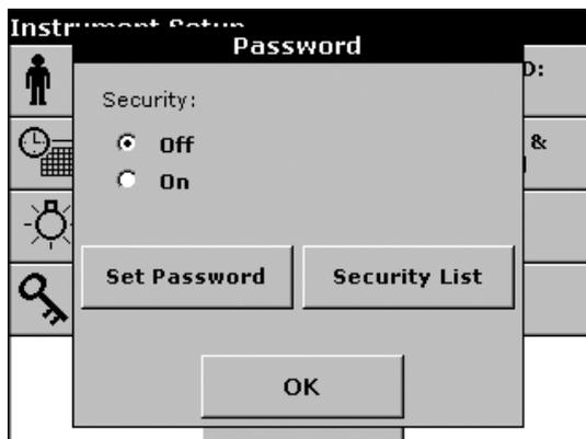
5. Activate the desired functions for which access is to be controlled (New ID, Delete ID, New Program, Edit Program, Delete Program, Update Software). Press **OK** to confirm and return to the Password menu.
