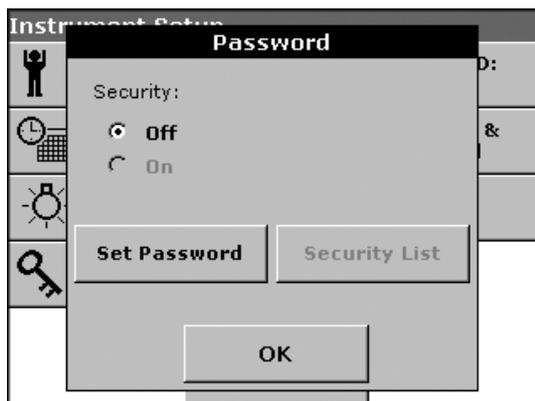
3. Use the alphanumeric keypad to enter a new password (up to 10 characters each), press **OK** to confirm. Access to the Security List is activated.
