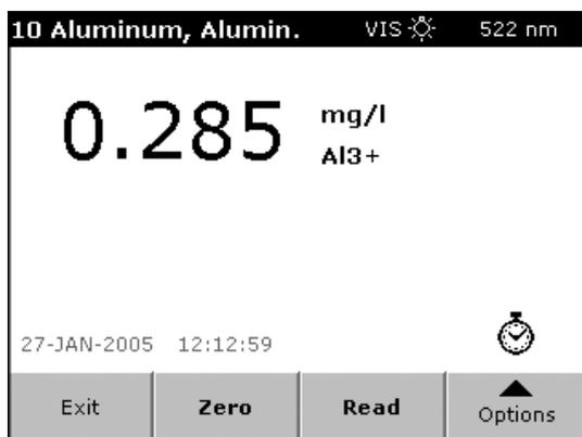
**Note:** If the Reading Mode is set to Single, press **READ** to obtain the result.
