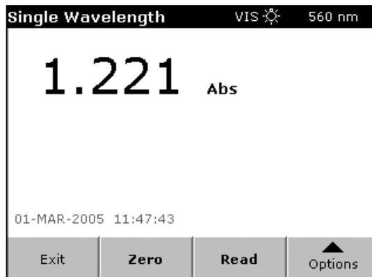
**Note:** The **READ** key is only active after the zero measurement has been completed.
