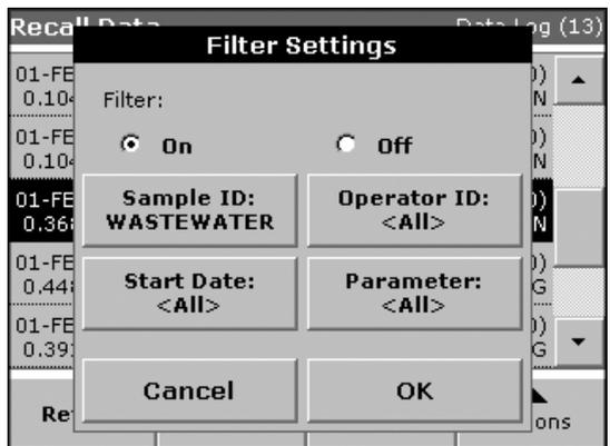
4. Select On to turn on the filters and select data by Sample ID, Operator ID, Start Date, Parameter, or any combination of the four.
