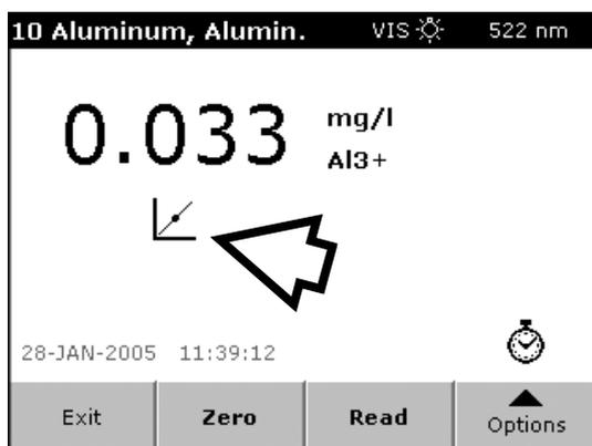
**Note:** The adjustment must be within certain limits, which vary with each program. The allowable percentage is shown after "Adjustment >"
