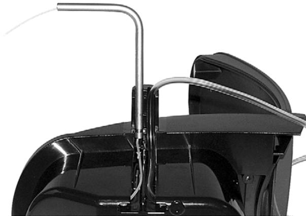
3. Hold the rubber fitting with the ridges over the grooves and push it firmly onto the guide tube and the waste tube. The rubber fitting must firmly enclose the guide tube and drain tube.
