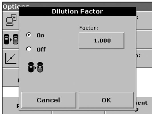
3. Press **OK** to confirm. Press **OK** again. When a dilution is in effect, the Dilution icon will appear on the display.
