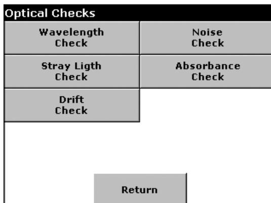
2. Select the type of optical check to perform (wavelength, noise, stray light, absorbance, or drift).
