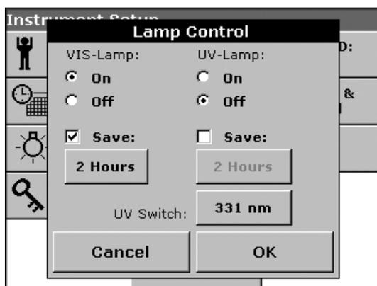
2. Select On to toggle on the VIS-Lamp or UV-Lamp, respectively.
