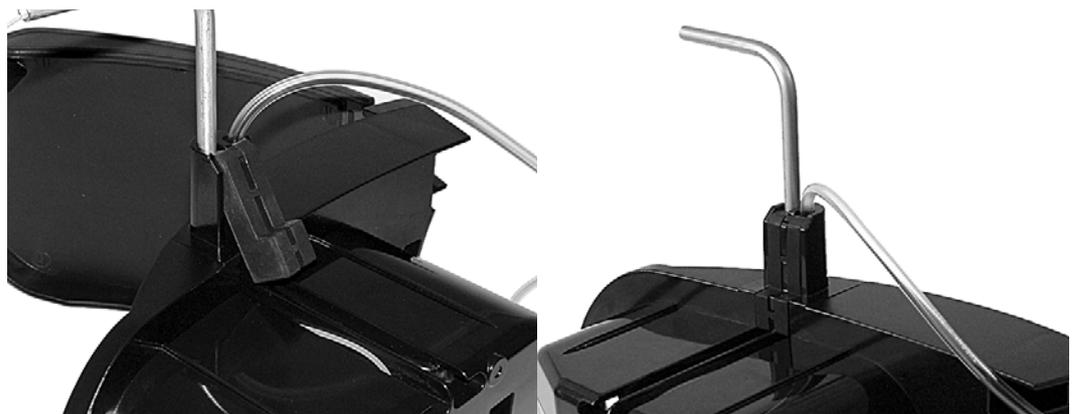
4. Open the cell compartment. Without the locking screws, insert the Multi Cell Holder into the cell compartment (refer to [section 3.4.1 on page 14](#)).
