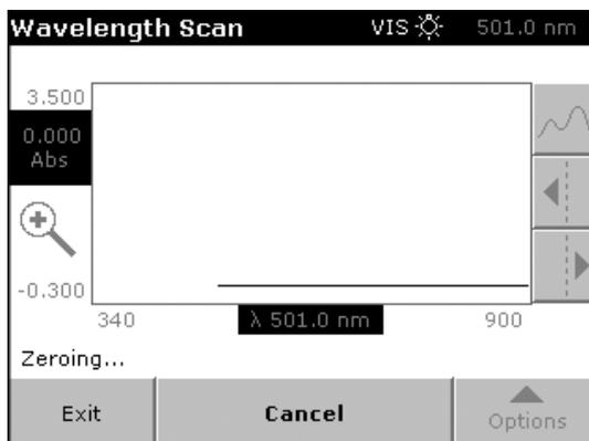
**Note:** The UV lamp is not switched on until a wavelength in the UV spectrum has been entered and the blank reading has been started. In the warm-up phase of the UV lamp, the message "Warming up..." is displayed and the icon UV lamp flashes. As soon as the UV lamp is ready, the blank reading is performed.
