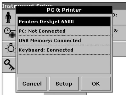
2. Press **PRINTER** and then press **SETUP** to display the Printer Setup screen. The Printer Setup screen allows the user to set the resolution and paper size.
