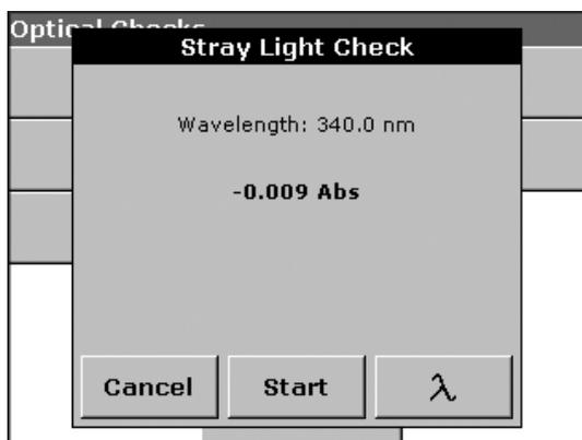
6. The result will be displayed. Thirty readings are averaged for the blank. The Average and Standard Deviation are calculated from 100 consecutive absorbance readings. The Average of the readings is the stray light value in absorbance.
