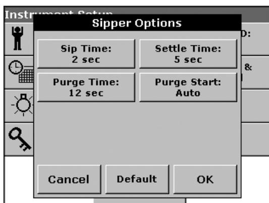
Press **ZERO** or **READ** to run the programs through the sipper cycles automatically. Press **READ** to run the program through the Sipper Module.
