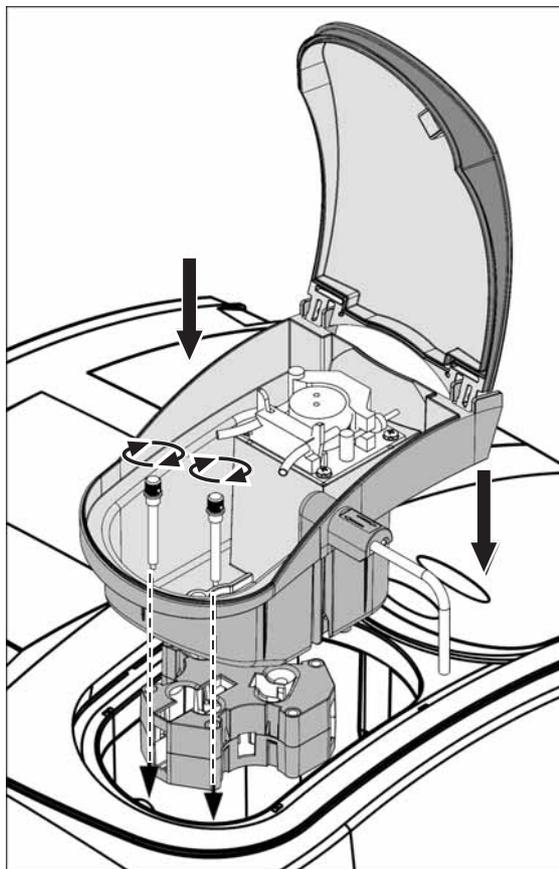
6. Secure the Sipper Module and the Multi Cell Holder with the two locking screws ([Figure 9 on page 121](#)).
