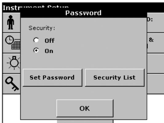
4. Press **OK** to deactivate the former password and return to the Password menu. Set a new password, refer to [section 5.2.7 on page 27](#).
