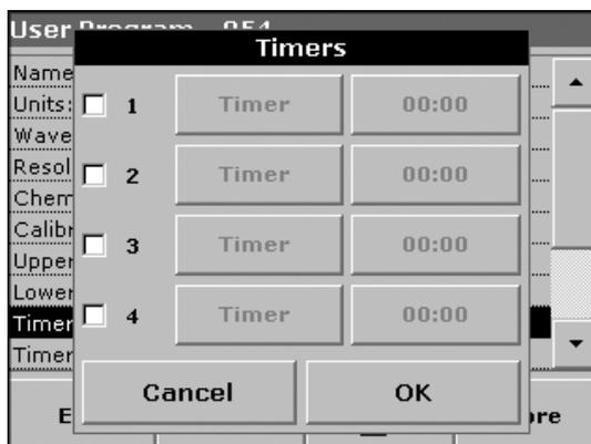
3. Check the appropriate timer(s). Press the **TIMER** key to select from a list of names that describe the corresponding step. Press **00:00** to enter the times for each timer.
