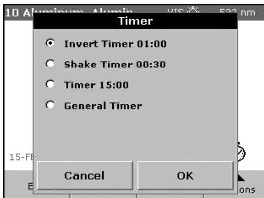
1. Press the **TIMER** (clock) icon on the display. Press **OK** to start the timer. The timer will count down on the screen.
