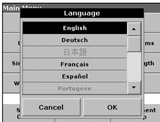
Once the language is selected, the instrument continues to power up in that language until a different language is selected. To change the language after initial installation, press any area of the display with the instrument off. Turn the instrument on, continue to press the display until the list of languages is displayed.
