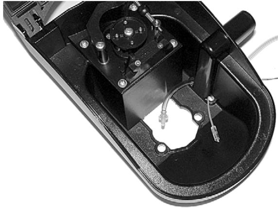
2. Turn the sipper module on its side. Pull the inlet tube and the drain tube through, respectively, the entry channel and the exit channel of the sipper. The inlet tube must be pulled through the guide tube. The bottom end of the guide tube must click into the channel. Avoid kinks in the tubes.
