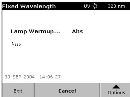
When the lamp is warm and ready, the UV Lamp icon stops flashing. If both lamps are on, the UV-VIS icon is displayed in the selected Measurement Mode.
