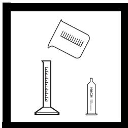
**1.** Select the sample volume and Sodium Thiosulfate Titration Cartridge corresponding to the expected chlorine concentration from *Table 1*.
