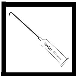
**1.** Insert a clean delivery tube into the Magnesium Chloride Titration Cartridge. Attach the cartridge to the titrator body. See *General Description, Step-By-Step*, for assembly instructions.
