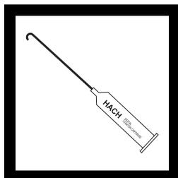
**2.** Insert a clean delivery tube into the titration cartridge. Attach the cartridge to the titrator body. See *General Description Section, Step-by-Step*, for assembly instructions if necessary.
