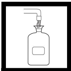
**1.** Collect a water sample in a clean 300-mL BOD Bottle.
