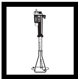
6. Place the delivery tube tip into the solution and swirl the flask while titrating with mercuric nitrate from a yellow to light pink color. Record the number of digits required.
