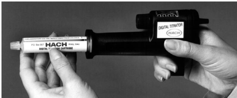
3. Remove the polyethylene cap and insert a clean delivery tube into the end of the cartridge until it is tight. See *Figure 3*. Use a straight tube with a hook at the end for hand-held titrations; use a 90° tube with a hook at the end for stationary setups.
