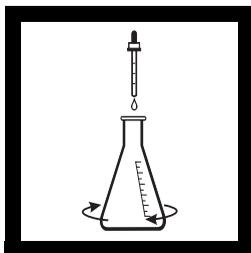
10. Add one dropper of Starch Indicator Solution to the flask and swirl to mix. A dark blue or green color will develop.
