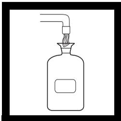
**1.** Collect a water sample in a clean 60-mL glass-stoppered BOD Bottle.
