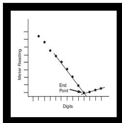
$$\begin{aligned} &\text{Digits at} \\ &\text{End Point} \times 1.25 \\ &= \mu\text{g/L Free Chlorine} \\ &\text{as Cl}_2 \end{aligned}$$
