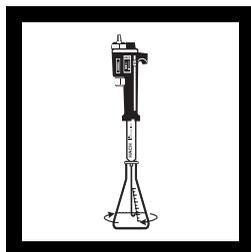
6. Place the delivery tube tip into the solution and swirl the flask while titrating with sodium hydroxide until a light pink color forms and persists for 30 seconds. Record the number of digits required.
