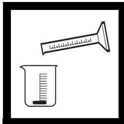
**3.** With minimum agitation, measure 200 mL sample with a clean graduated cylinder and transfer the sample to the beaker. Swirl to mix the reagents with sample.
