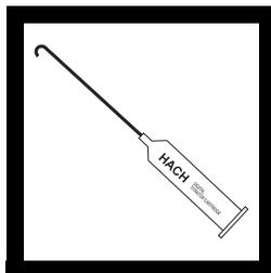
**7.** Attach a clean straight-stem delivery tube to a 0.2000 N Sodium Thiosulfate Titration Cartridge. Twist the cartridge onto the titrator body. See General Description, Step-by-Step for assembly instructions, if necessary
