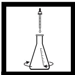
**5.** Add five drops of 5.25 N Sulfuric Acid Standard Solution to the flask. Swirl to mix.
