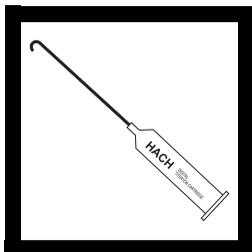
**1.** Insert a clean delivery tube into the Bismuth Nitrate Titration Cartridge. Attach the cartridge to the titrator body. See *General Description, Step-By-Step*, for assembly instructions.
