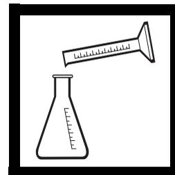
**4.** Use a graduated cylinder or pipet to measure the sample volume from *Table 1*. Transfer the sample to a clean 125-mL Erlenmeyer flask. Dilute to about the 50-mL mark with deionized water.
