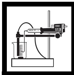
7. Using the Digital Titrator delivery knob, dispense the Standard Iodine Titrant Solution in 5-10 digit increments while noting the LED reading. Record at least 3 points (null current values and Digital Titrator reading), before end point is reached.
