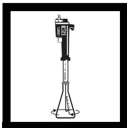
**10.** Place the delivery tube tip into the solution and swirl the flask while titrating with sodium thiosulfate to a pale yellow color.
