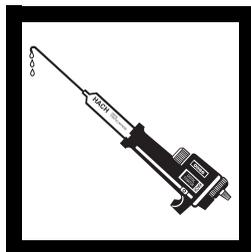
**2.** Hold the Digital Titrator with the cartridge tip pointing up. Turn the delivery knob until a few drops of titrant are expelled. Reset the counter to zero and wipe the tip.
