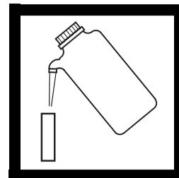
**4.** Fill the vial to the 10-mL mark with deionized water.
