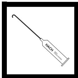
**2.** Attach a clean delivery tube to a 0.9274 N Sodium Hydroxide titration cartridge. Attach the cartridge to the titrator body. See *General Description, Step-by-Step*, for assembly instructions, if necessary.
