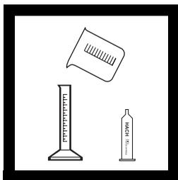
**1.** Select a sample volume and a Sodium Hydroxide (NaOH) Titration Cartridge corresponding to the expected acidity concentration as mg/L calcium carbonate (CaCO<sub>3</sub>) from *Table 1*.
