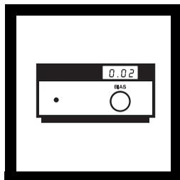
6. Note the LED reading on the Amperometric Titrator. It should read  $0.00 \pm 0.05$ . DO NOT adjust the BIAS control.
