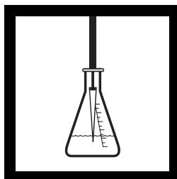
**7.** Use the pipet to dispense 0.2 mL of bleach sample below the solution level in the flask.
