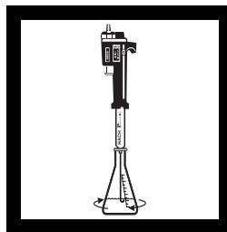
**7.** Place the delivery tube tip into the solution. While swirling the flask, titrate with the Bismuth Nitrate until the color changes from yellow to blue-green. Record the number of digits required.
