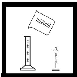
1. Select the sample volume corresponding to the expected acid concentration in milliequivalents (meq)/L or normality (N) from *Table 1*.
