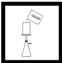
**6.** Pour a total of about 800 mL, in three portions, of deionized water through the filter funnel and wait until it passes through the filter. Discard this rinse water.
