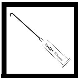
**1.** Insert a clean delivery tube into the 8.00 N Sulfuric Acid Titration Cartridge. Attach the cartridge to the titrator body.
