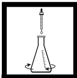
**6.** Add one drop of Ferroin Indicator Solution to the flask. Swirl to mix.
