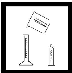
1. Select the sample volume corresponding to the expected base concentration in milliequivalents/L or normality from *Table 1*.
