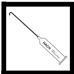
**1.** Insert a clean delivery tube into the 2.26 N Thiosulfate Titrant Solution cartridge. Attach the cartridge to the titrator body.
