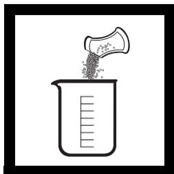
5. Add the contents of one pillow of Potassium Iodide Reagent to the beaker and allow the powder to dissolve.
