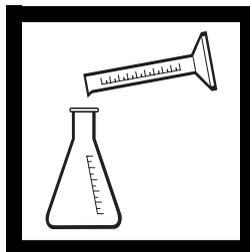
**3.** Use a graduated cylinder to measure the 100 mL of sample into a 125-mL Erlenmeyer flask.
