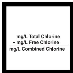
**7.** If total residual chlorine is desired, return to *step 3* and substitute a DPD Total Chlorine Powder Pillow in *step 4*. Wait three minutes before titrating. Continue with *step 5*. The results will be expressed as mg/L total chlorine.
