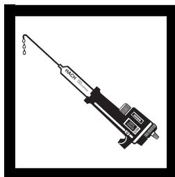
**2.** Install the 0.00564 N Phenylarsine Oxide (PAO) cartridge. Flush the Digital Titrator delivery tube by turning the delivery knob to eject a few drops of titrant. Reset the counter to zero and wipe the tip.
