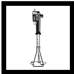
6. Place the delivery tube tip into the solution and swirl while titrating with sodium hydroxide until a light pink color appears. Record the number of digits required.
