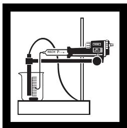
6. Place the beaker on the TitraStir® Stir Plate and immerse the tips of the probe and delivery tube in the solution. The probe's platinum wires must be submerged. Turn on the stirring motor.
