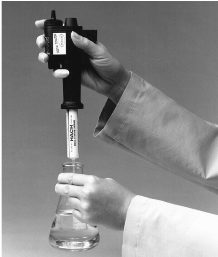
6. Use the smallest appropriate graduated cylinder or pipet to measure the sample volume from the given table. Transfer the sample into a 125-mL or 250-mL Erlenmeyer flask. Dilute to the appropriate total volume with deionized water if necessary.
