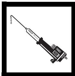
**2.** Turn the delivery knob to eject a few drops of titrant. Reset the counter to zero and wipe the tip.
