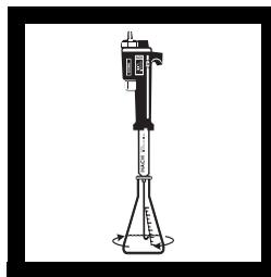
**7.** Place the delivery tube tip into the solution and swirl the flask while titrating with the iodate-iodide to a permanent blue end point. Record the number of digits required.
