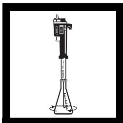
**5.** Place the delivery tube tip into the solution and swirl the flask while immediately titrating with FEAS to a colorless end point. Record the number of digits required.
