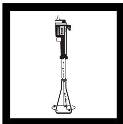
6. Titrate with 8.00 N hydrochloric acid or sulfuric acid until the solution is colorless. Record the number of digits required.
