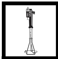
**7.** Place the delivery tip into the solution. While titrating with Ceric Standard Solution, swirl the flask until the solution color changes from orange to pale blue. Record the number of digits required.
