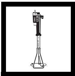
**9.** Place the delivery tube tip into the solution. Swirl the flask while titrating with the sulfuric acid titrant until the solution color changes from purple to orange-red. Record the number of digits used.
