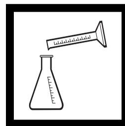
4. Use a graduated cylinder or pipet to measure the sample volume from Table 2. Transfer the sample into a clean 250-mL Erlenmeyer flask. Dilute to about the 100-mL mark with deionized water, if necessary.
