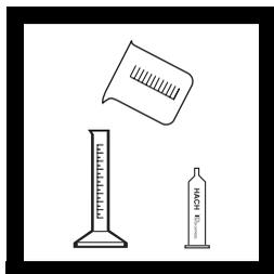
**1.** Select the sample volume and Sodium Thiosulfate Titration Cartridge corresponding to the expected chlorine concentration from *Table 2*.
