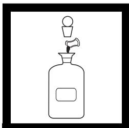
**5.** Remove the stopper and add the contents of one Sulfamic Acid Powder Pillow. Replace the stopper without trapping air in the bottle and invert several times.
