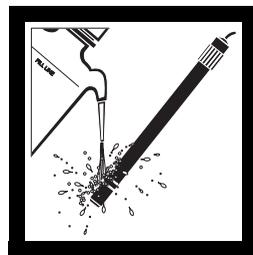
5. Place the beaker on the TitraStir® Stir Plate and immerse the tips of the probe and delivery tube in the solution. The probe's platinum wires must be submerged. Turn on the stirring motor.
