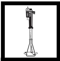
$$\begin{array}{l} \text{Digits} \\ \text{Required} \times 0.1 \\ = \text{mg/L Dissolved Oxygen} \end{array}$$
