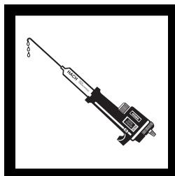
**3.** Turn the delivery knob to eject a few drops of titrant. Reset the counter to zero and wipe the tip.
