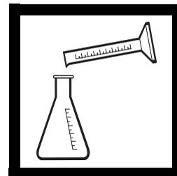
**4.** Use a graduated cylinder or pipet to measure the sample volume from *Table 1*. Transfer the sample to a clean 125-mL Erlenmeyer flask. Add deionized water to about the 75-mL mark, if necessary.
