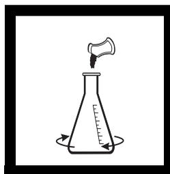
**11.** Add the contents of one ManVer® 2 Hardness Indicator Powder Pillow (Cat. No. 928-99) or 4 drops of Hardness 2 Test Solution (Cat. No. 425-32). Swirl to mix.
