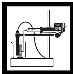
7. Using the Digital Titrator delivery knob, dispense the PAO titrant Solution in 5-10 digit increments while noting the LED reading.
