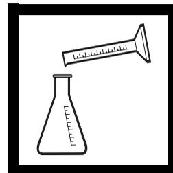
**4.** Select the distillate volume corresponding to the expected volatile acids concentration as acetic acid from *Table 1*. Using a graduated cylinder, transfer the distillate volume into a clean 250-mL Erlenmeyer flask and dilute to about the 150-mL mark with deionized water.
