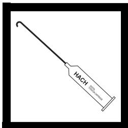
**1.** Insert a clean delivery tube into the Sodium Thiosulfate titration cartridge. Attach the cartridge to the titrator body. See *General Description, Step-by-Step*, for assembly instructions, if necessary.
