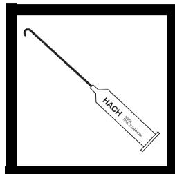
**2.** Insert a clean delivery tube into the titration cartridge. Attach the cartridge to the titrator body. See *General Description, Step-by-Step* for assembly instructions, if necessary.
