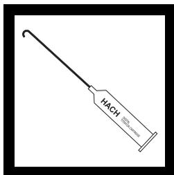
2. Insert a clean delivery tube into the appropriate Hydrochloric Acid or Sulfuric Acid Titration Cartridge. Attach the cartridge to the titrator body. See *General Description Section, Step-by-Step*, for assembly instructions, if necessary.
