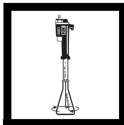
**7.** Place the delivery tube tip into the solution and swirl the flask while titrating with EDTA from red to pure blue. Record the number of digits required.
