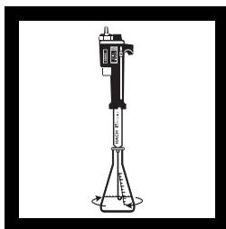
**6.** Place the delivery tube tip into the solution and swirl the flask while titrating with silver nitrate from a yellow to red-brown color. Record the number of digits required.
