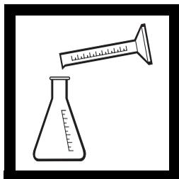
**9.** Use a graduated cylinder to measure the sample volume from *Table 1*. Transfer the sample into a 250-mL Erlenmeyer flask.
