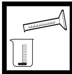
**3.** With minimum agitation, measure 200 mL sample with a clean graduated cylinder. Transfer the sample to a clean 250-mL beaker containing the 50-mm stirring bar supplied with the system.
