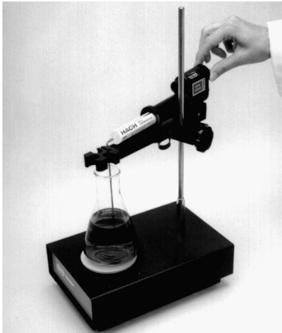
Figure 5 Using a Laboratory Stand
