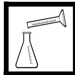
4. Use a graduated cylinder or pipet to measure the sample volume from *Table 1*. Transfer the sample into a clean 125-mL Erlenmeyer flask. Dilute to about the 50-mL mark with deionized water.
