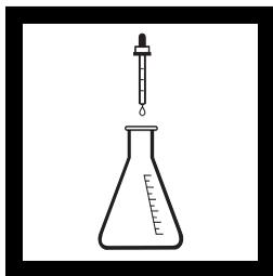
**6.** If the solution in the flask is yellow, add one drop of 5.25 N Sulfuric Acid Standard Solution. If the solution is blue, add 5.25 N Sulfuric Acid Standard Solution dropwise until the solution changes to yellow. Add one additional drop.
