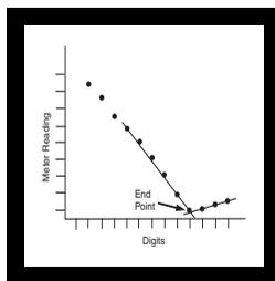
**11.** Using linear graph paper, plot the recorded readings from the Amperometric Titrator on the vertical axis and the corresponding Digital Titrator digits on the horizontal axis. Draw the two best intersecting lines through the points see *Figure 1*. Determine the number of digits at the intersection of the lines; this is the end point.
