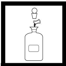
**5.** Remove the stopper and add the contents of one Dissolved Oxygen 3 Powder Pillow. Replace the stopper without trapping air in the bottle and invert several times to mix.
