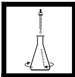
**11.** Add two 1-mL droppers of Starch Indicator Solution and swirl to mix.
