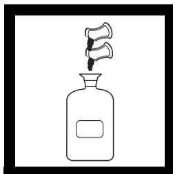
**2.** Add the contents of one Manganous Sulfate Powder Pillow and one Alkaline Iodide-Azide Reagent Powder Pillow.
