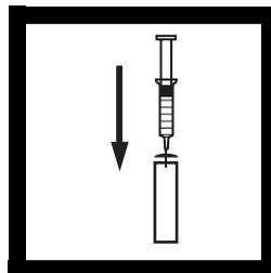
**3.** Using the 3-mL (3-cc) syringe, collect a 2.0-mL water sample. Add to the vial provided.
