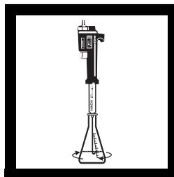
**7.** Place the delivery tube tip into the solution and swirl the flask while titrating with EDTA from pink to blue. Record the number of digits required.
