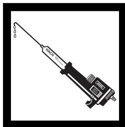
**2.** Flush the delivery tube by turning the delivery knob to eject a few drops of titrant. Reset the counter to zero and wipe the tip.
