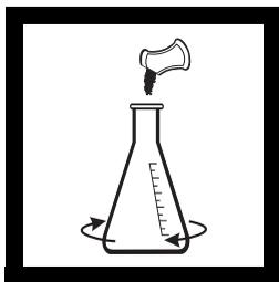
6. Clip open the end of one Potassium Iodide Powder Pillow. Add the contents to the flask. Swirl to mix.
