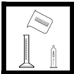
**1.** Select a sample size and an EDTA Titration Cartridge corresponding to the expected total hardness as calcium carbonate (CaCO<sub>3</sub>) concentration. Use *Table 1* for concentrations in mg/L or *Table 2* for concentrations in German degrees of hardness (G.d.h.).
