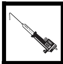
**3.** Hold the Digital Titrator with the cartridge tip pointing up. Turn the delivery knob until a few drops of titrant are expelled. Reset the counter to zero and wipe the tip.
