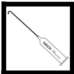
**1.** Insert a clean, straight-stem delivery tube to a Mercuric Nitrate Titration Cartridge. Attach the cartridge to the titrator body. See *General Description, Step-by-Step* for assembly instructions, if necessary.
