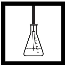
**6.** Dispense the sample below the liquid level in the flask. Dispense another 100  $\mu$ L of sample into the flask (200  $\mu$ L sample size). For other sample sizes, repeat until the required sample volume from step 4 has been added.
