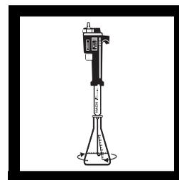
**12.** Place the delivery tube tip into the solution and swirl the flask while titrating with EDTA from red to pure blue. Record the number of digits required.
