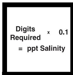
**7.** Determine the salinity of the water sample in parts per thousand (ppt) by multiplying the reading by 0.1.
