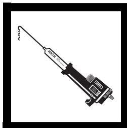
**2.** Flush out the delivery tube by turning the knob until titrant begins flowing from the end of the tube. Wipe the tip and reset the counter to zero.
