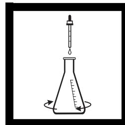
**4.** Using the 1-mL calibrated dropper, add 2 mL of Hardness 1 Buffer Solution to the flask and swirl to mix.
