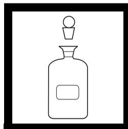
**3.** Immediately insert the stopper so air is not trapped in the bottle. Invert several times to mix.
