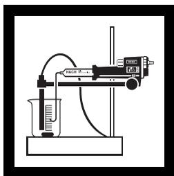
**10.** Continue the titration, recording at least three points on the downward sloping curve and at least three points after the end point has been reached. The latter points will have little change in the LED readings.
