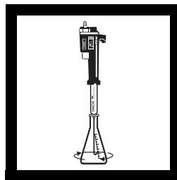
7. Place the delivery tube tip into the solution and swirl the flask while titrating with sodium thiosulfate to a straw-yellow color.
