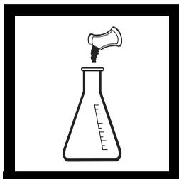
5. Add the contents of one Phenolphthalein Indicator Powder Pillow and swirl to mix. The solution should be colorless.
