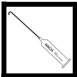
**1.** Insert a clean delivery tube into a 0.00564 N Ferrous Ethylenediammonium Sulfate (FEAS) Titration Cartridge. Attach the cartridge to the titrator body. See *General Description, Step-by-Step*, for assembly instructions, if necessary.
