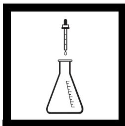
**9.** After completing the calcium titration, add 1 mL of 5.25 N Sulfuric Acid Standard Solution. Add additional acid dropwise and swirl the solution until the color changes from pure blue to purple, then to blue and finally to red. Swirl the flask to ensure that all precipitated magnesium hydroxide has re-dissolved.
