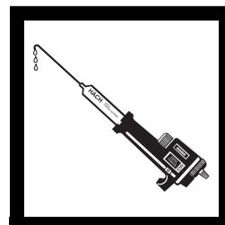
**8.** Turn the delivery knob to eject a few drops of titrant. Reset the counter to zero and wipe the tip.
