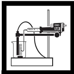
**2.** Install the Standard Iodine Titrant Cartridge, 0.028 N. Flush the Digital Titrator delivery tube by turning the delivery knob to eject a few drops of titrant. Reset the counter to zero and wipe the tip.
