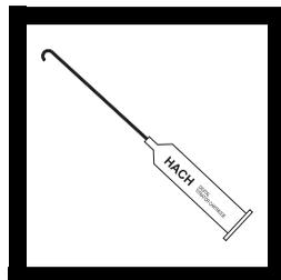
2. Insert a clean delivery tube into the Iodate-Iodide Titration Cartridge ( $\text{KIO}_3\text{-KI}$ ). Attach the cartridge to the titrator body. See *General Description, Step-by-Step*, for assembly instructions, if necessary.
