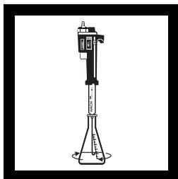
**6.** If the solution turns pink, titrate to a colorless end point. Place the delivery tube tip into the solution and swirl the flask while titrating with sulfuric acid. Record the number of digits required.
