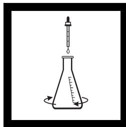
**7.** Add 1 mL (one full dropper) of Wide Range pH Indicator Solution to the flask.
