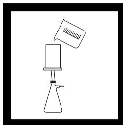
**7.** Again add 800 mL of deionized water through the filter funnel and collect in a filter flask. Remove vacuum hose from sidearm and turn off water.
