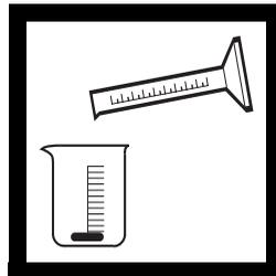
**3.** Using a graduated cylinder, measure 200 mL of deionized water into a clean 250-mL beaker. Place the 50-mm stirring bar supplied with the system into the beaker.
