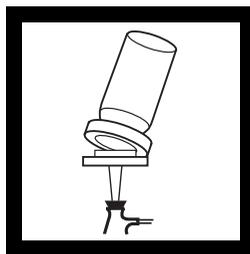
**3.** Cover the stem with the filter housing.
