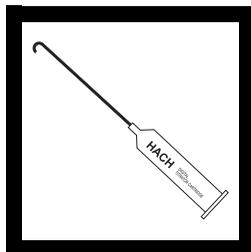
2. Insert a clean delivery tube into the appropriate Sodium Hydroxide Titration Cartridge. Attach the cartridge to the titrator body. See *General Description, Step-by-Step*, for assembly instructions.
