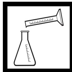
**4.** Use a pipet or graduated cylinder to measure the sample volume from *Table 2*. Transfer the sample into a 125-mL Erlenmeyer flask and dilute to about the 50-mL mark with deionized water.
