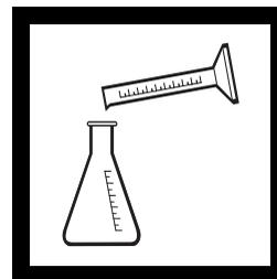
4. Use a graduated cylinder or pipet to measure the sample volume from *Table 1*. Transfer the sample into a clean 250-mL Erlenmeyer flask. Dilute to about the 100-mL mark with deionized water, if necessary.
