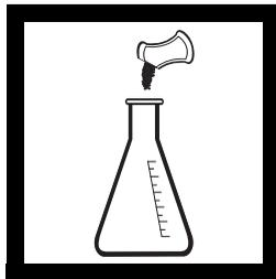
**6.** If you are using the 2.00 N titration cartridge, add the contents of one Potassium Iodide Powder Pillow (Cat. No. 20599-96) to the flask and swirl to mix.
