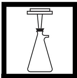
**1.** Attach the filter funnel stem to a 1000-mL filtering flask.
