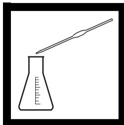
**3.** Pipet 25.0 mL of sample into a 50-mL Erlenmeyer flask.
