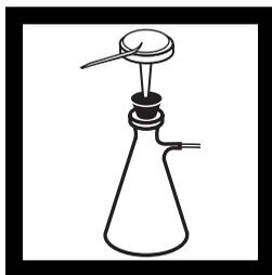
**2.** Using plastic tweezers, position a 0.45 micron membrane filter on top of the funnel stem.
