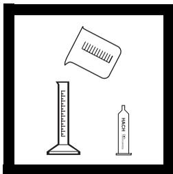
**1.** Select a sample size and a Sodium Hydroxide (NaOH) Titration Cartridge corresponding to the expected carbon dioxide (CO<sub>2</sub>) concentration; see *Table 1*.
