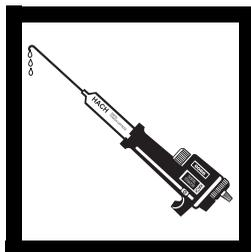
**2.** Flush the delivery tube by turning the deliver knob to eject a few drops of titrant. Reset the counter to zero and wipe off the tip.
