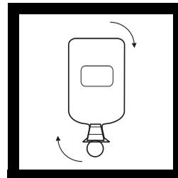
**4.** Wait until the floc in the solution has settled and the top half of the solution is clear. Again invert the bottle several times and wait until the floc has settled.
