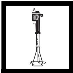
**6.** Place the delivery tube tip into the solution and swirl the flask while titrating with sodium hydroxide from yellow to blue-violet (pH 3.7). Record the number of digits required.
