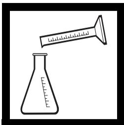
1. Measure a second portion of the sample selected from *step 1 on page 35* into a clean 250-mL Erlenmeyer flask. Dilute to about the 100-mL mark with deionized water, if necessary.
