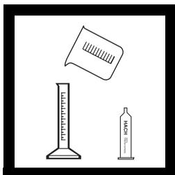
**1.** Select the sample volume and Mercuric Nitrate Titration Cartridge corresponding to the expected chloride concentration from *Table 1*.
