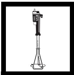
9. Place the delivery tube tip into the solution and swirl the flask while titrating with the thiosulfate titrant until the solution is pale yellow.
