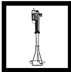
**7.** Place the delivery tube tip into the solution and swirl the flask while titrating with sodium thiosulfate until the solution is a pale yellow.
