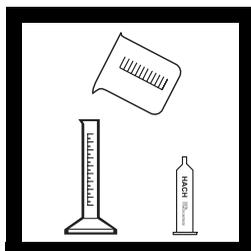
**6.** Select a sample volume and Sodium Thiosulfate Titration Cartridge corresponding to the expected dissolved oxygen (D.O.) concentration from Table 1.
