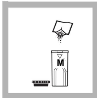
6. Add the contents of one pillow of Monochlor F to the cell for Monochloramine measurement.
