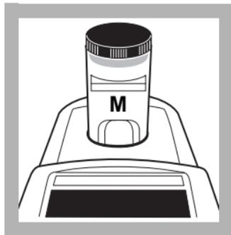
3. Place the cell for Monochloramine measurement into the cell holder.
