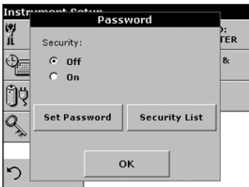
4. Press **SECURITY LIST** to lock various functions for unauthorized users.
