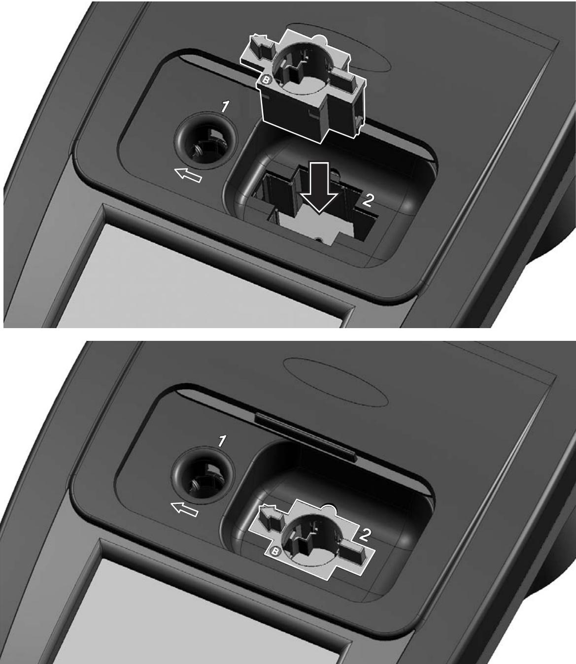
Figure 5 Installing a Cell Adapter
