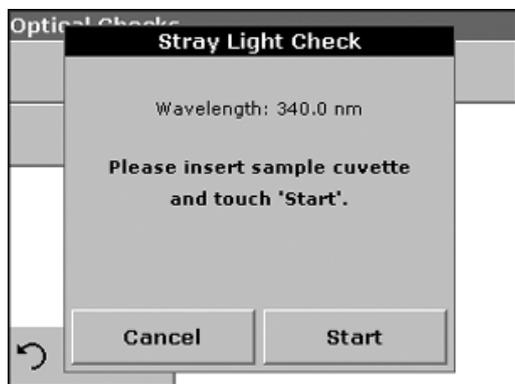
4. Insert the sample cell into the Cell Compartment #2. Close the cell compartment. Press **START**.
