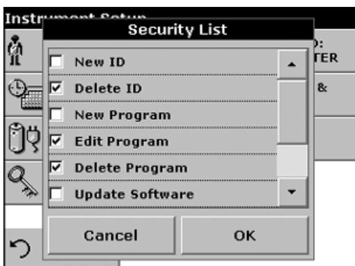
5. Activate the desired functions to control. Press **OK** to confirm the Security List. The Password menu will be displayed.
