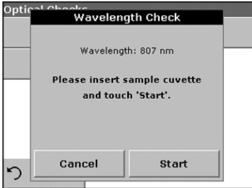
The Wavelength Check test is used to check wavelength accuracy at 807 nm. The wavelength check requires the Filter Set (Cat. No. LZV537).
