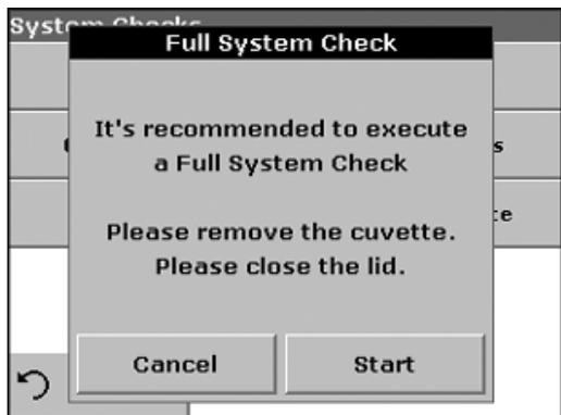
If the instrument detects any deviation relative to the last calibration, it is recommended to perform a system check.
