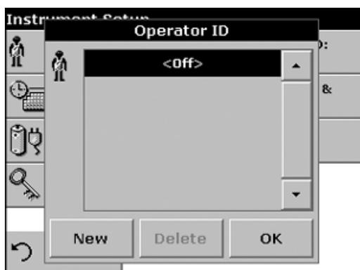
Use this option to enter up to 30 sets of operator initials (up to five characters each) into the instrument. This feature helps record which operator measured each sample.
