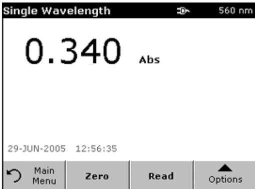
1. Insert the blank cell into the cell holder. Press **ZERO**.
