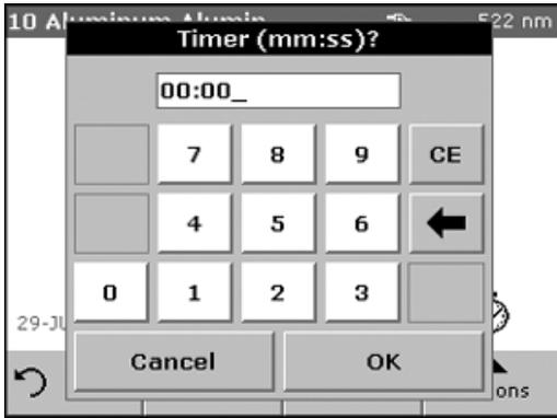
A general purpose timer is also available in many programs. When the timer icon is visible, press the icon and select **GENERAL TIMER**. A new screen will appear. Enter the length of the timed interval and press **OK** to start the timer. The timer will beep when the timed interval ends.
