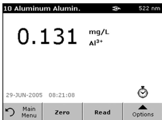
4. Remove zero solution cell and insert sample cell into the cell compartment. Press **READ**. The result will be displayed.
