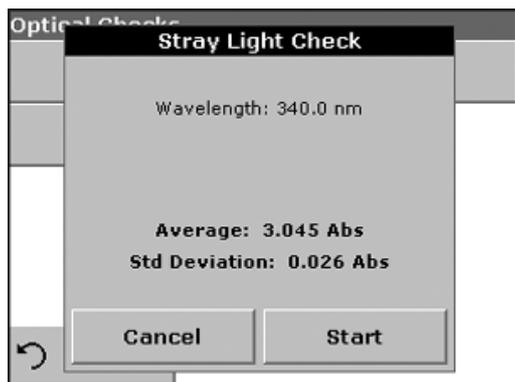
5. The Average and Standard Deviation are calculated from three successive absorbance measurements. The result is displayed and is to be compared with the nominal data of the sample cell.
