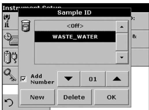
Use this option to enter up to 30 Sample Identification tags (up to 13 characters each) into the instrument. Sample IDs can be used to specify the sample location or other sample specific information.
