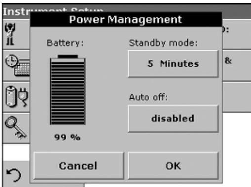
1. From Instrument Setup, press **POWER MANAGEMENT**. The battery symbol indicates the battery life in %.
