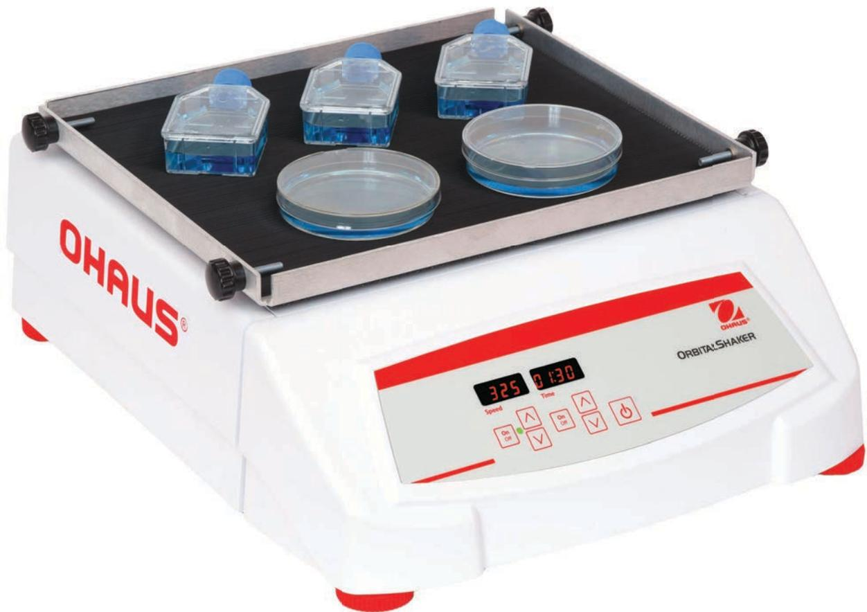
With load capacities from 16 to 68 kg and over 70 accessory options, OHAUS Heavy Duty Shakers are designed to handle a range of applications. Available as analog or digital models with microprocessor control to provide variable speed and consistent shaking, while ramping to the set speed. Microprocessor displays the last set-point and will restart if power is interrupted. Built-in tray and non-slip rubber mat included with all models.
