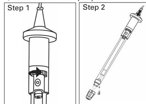
2) Press the spring loaded top and hold until as much liquid as possible leaks out of the junction near the pH glass.
