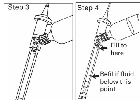
4) Please note also that the refill solution should not be allowed to drop 2.5" below the valve hole. If this occurs, add more solution until it reaches 1/2" under the refill hole of the ball-valve. Please use refill solution S20 or 3.5M KCl solution only. **NOTE: No other solution should be used!**
