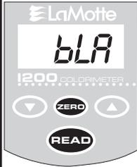
Push the **READ** button to turn the meter on. Press the **ZERO** button and hold it for 2 seconds until **BLA** is displayed. Release the button to take a zero reading (0.00 ppm).
