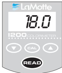
Align the index line with the arrow on the meter, insert tube into chamber. Close the lid. Push the **READ** button. Record results as ppm Fluoride.
