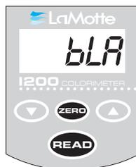
Push the **READ** button to turn the meter on. Press the **ZERO** button and hold it for 2 seconds until **bLA** is displayed. Release the button to take a blank reading (0.0 ppm).
