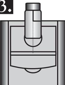
Insert the tube into the chamber, being sure to align the index line with the arrow on the meter. Close the lid. This tube is the sample blank or zero.
