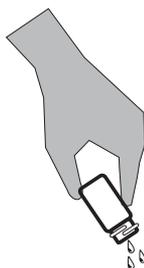
Rinse and fill a colorimeter tube (0290) to the 10 mL line with sample water. Cap and wipe dry.
