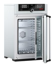
The heating of this incubator is optimally tuned for both natural convection and forced air circulation; the fan can also be switched off completely, and valuable chamber loads for research, pharmaceutics, medicine and food chemistry are warmed up very carefully.
